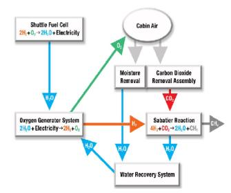
Fig. 3. NASA and ISS station model for produce essential material for astronauts (www.nasa.com).
