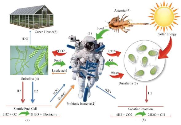
Fig. 2. Open and close bioreactor in space.
